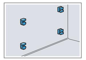
1. Hook the front retainers with the hook into the round hole at the top and set them at a slight angle ①.
