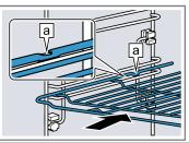
Baking tray Slide the tray in with the sloping E.g. univer- edge b towards the appliance door.
