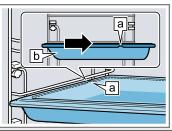
**3.** Push the accessory all the way in, making sure that it does not touch the appliance door.
