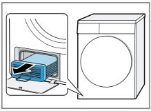
4. Clean the heat exchanger from all sides under running water and dry it.
